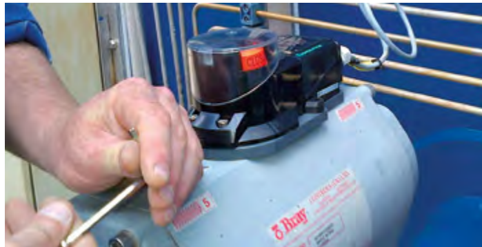
The F31K2 is easy to mount directly onto the pneumatic actuator. The sensor is directly attached to the drive housing, and the puck merely needs to be pushed onto the drive shaft and fixed in place according to the valve's current position.
